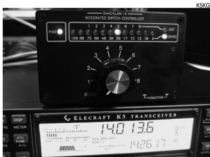
Figure 3 — Controller sitting atop an Elecraft K3, following the radio's frequency
