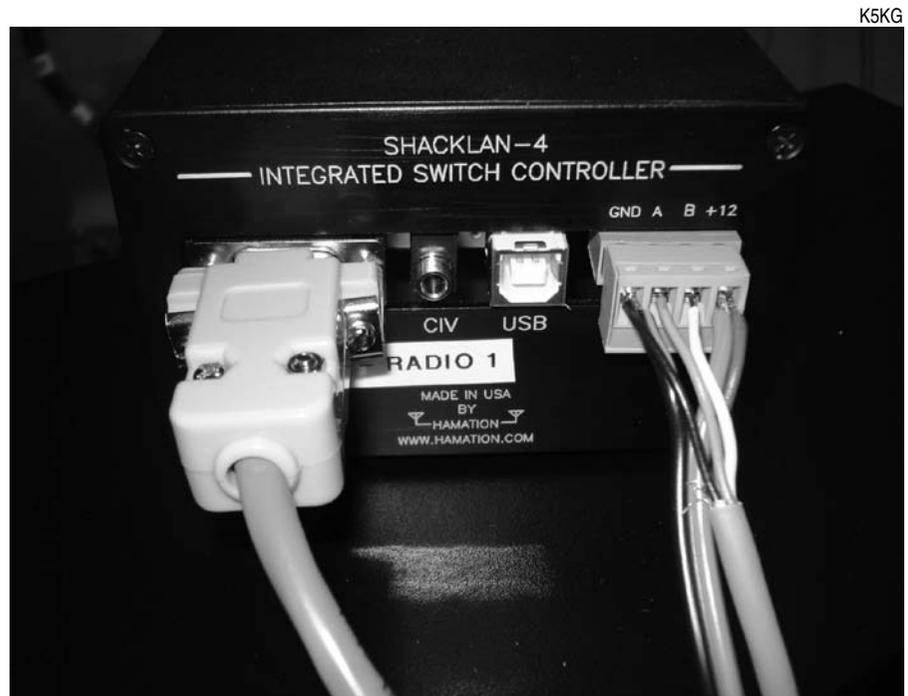
Figure 2 — ShackLAN-4 connector wiring detail
